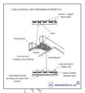
Lath and plaster ceiling overclad with plasterboard
