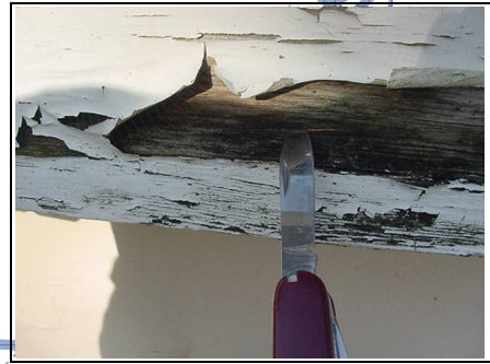
Knife test of timber
