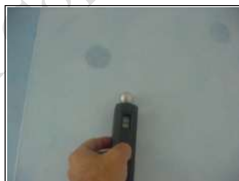
Testing for lateral dampness
