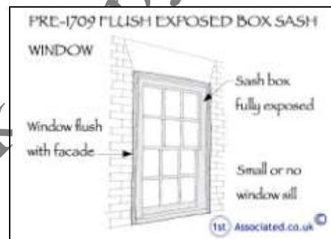
Pre-1709 exposed box sash window
