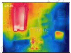
Left reception room with heat coming in through window and warmth of the radiator, with the blue being the coldness of the walls
